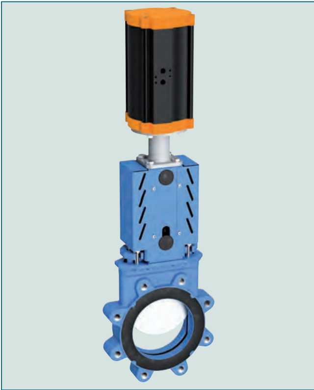
Knife Gate Valve with fully lugged body, which allows end of pipe installation.
